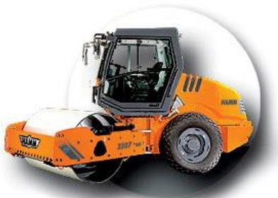
COMPACTEUR AVEC OSCILLATIONS ET VIBRATIONS
